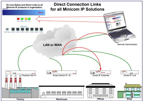
Figure 39 Direct connections link scenario
